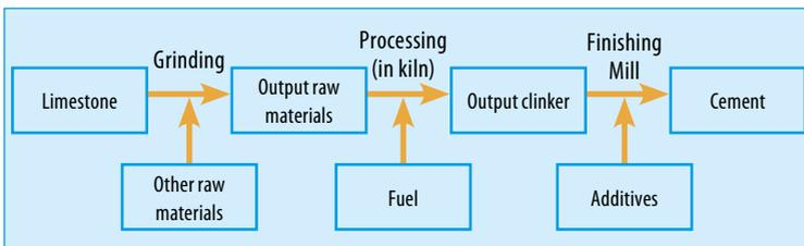
**Figure 2** – Main stages in cement production
