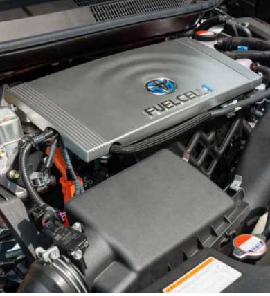
Engine of fuel-cell vehicle "Mirai" by Toyota.
