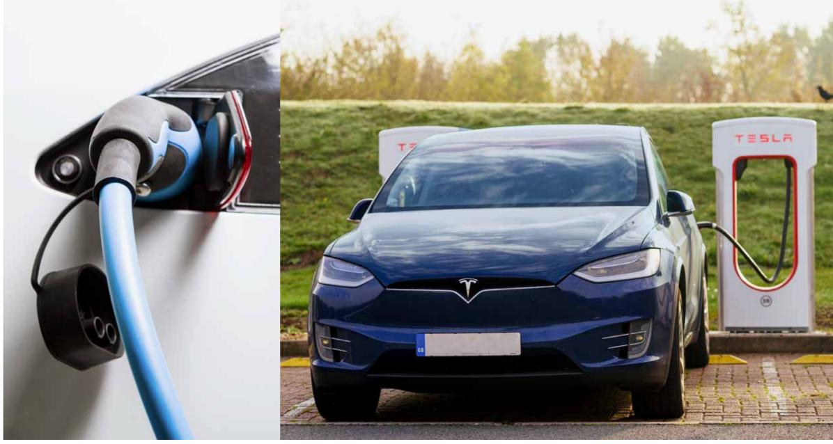
Electric vehicles must have a standard plug-in connector to charge from standard power points.
